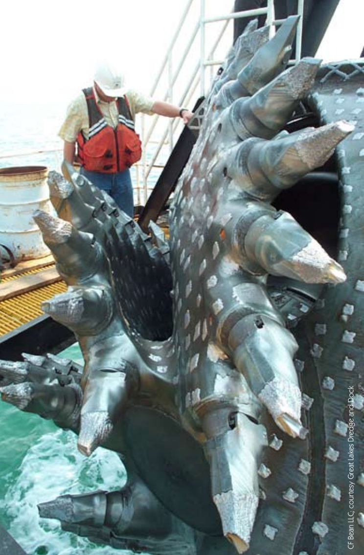
Above: As it spins, the massive cutterhead churns up sediment and directs it into a suction pipe.
