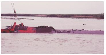
New technology, such as this plow, was used to form the low-level terraces by reforming bottom material from the bay.
