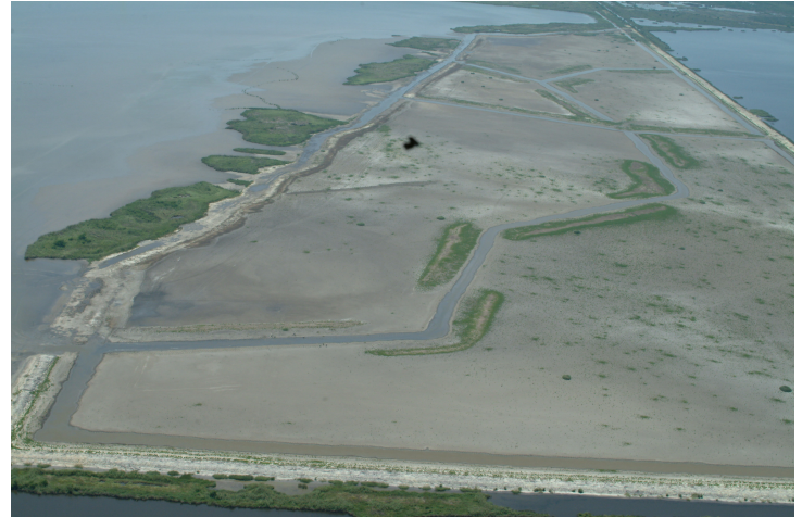
Sabine Marsh Creation Cycle I on Sabine NWR looking westward. Note the constructed trenasses for fisheries and water movement can be seen.
