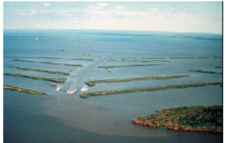
Aerial photo of constructed terraces in Little Vermilion Bay.
