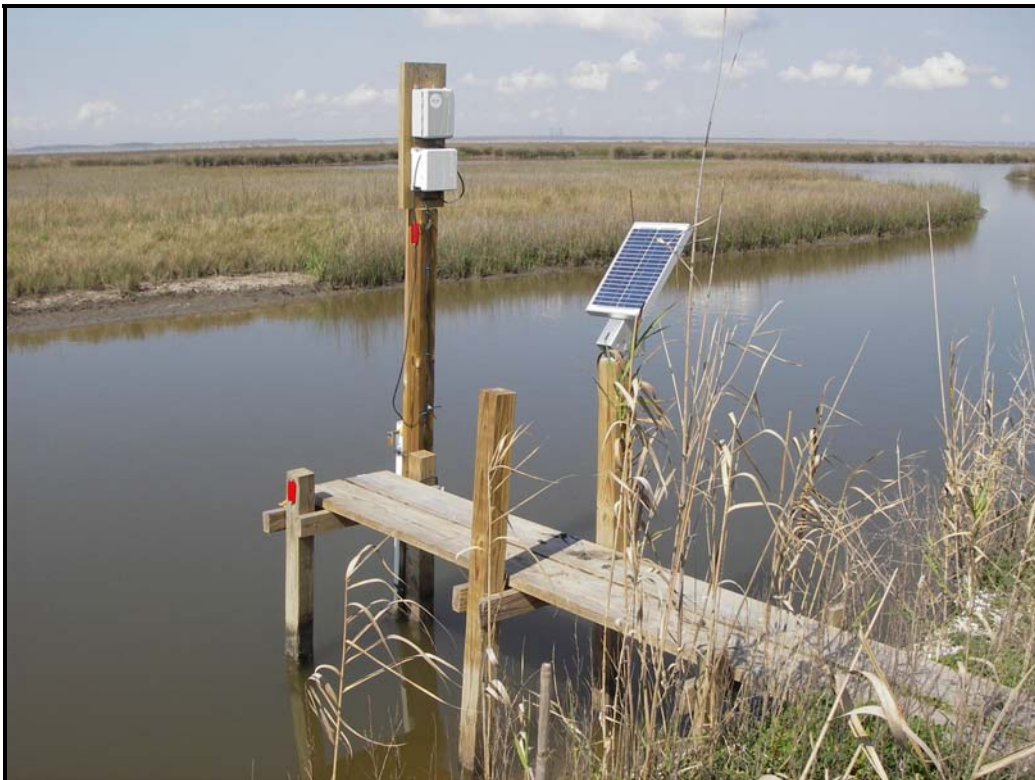
Photo 8. View showing Portable Multi-Parameter Water Quality Troll 9500 (15r) with wooden boardwalk near Structure No. 12. (March 8, 2007)
