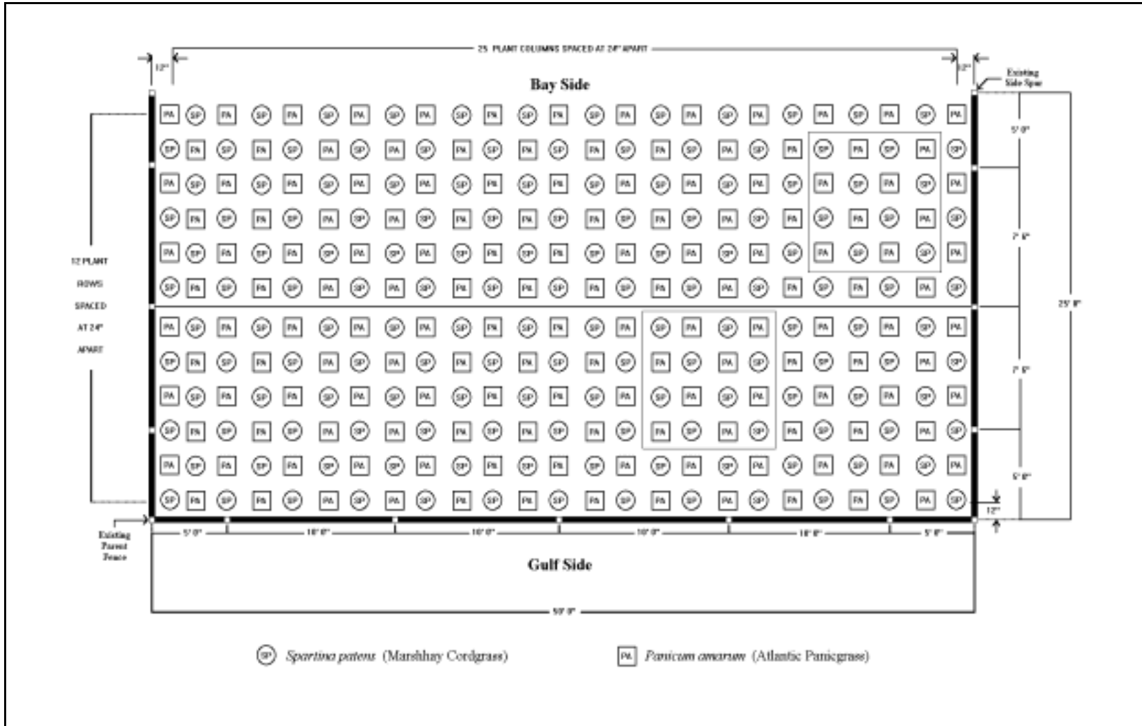
Figure 3. Typical layout for vegetation plantings within a 50 ft segment (fenced or unfenced) including randomly placed 2 m x 2 m vegetation plots at Timbalier Island Plantings (TE-18) Demonstration project.
