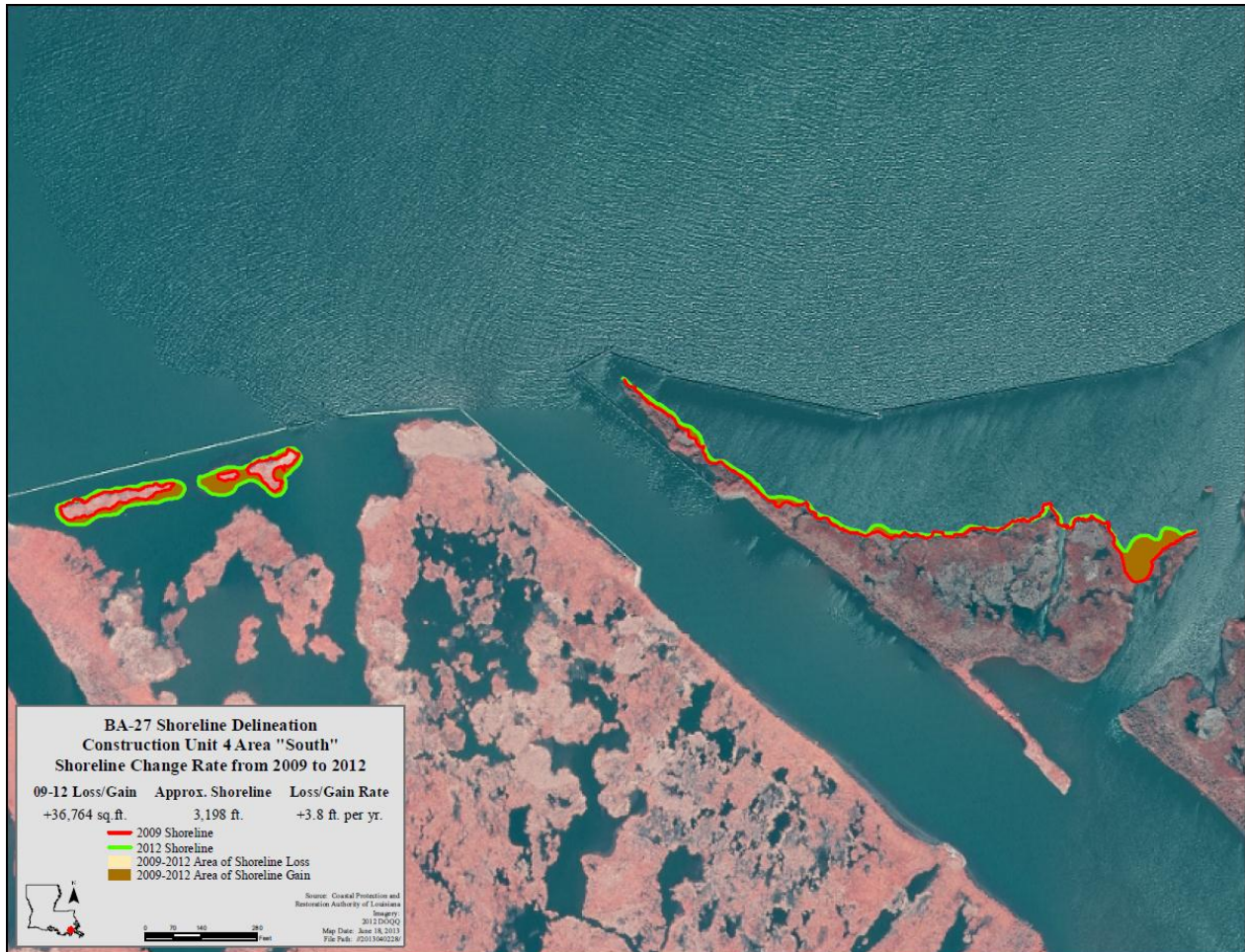
Figure 16. Post-construction shoreline change analysis for the southern section of Construction Unit 4 of the Barataria Basin Landbridge Shoreline Protection Project (BA-27c, Phase 3) from 2009 to 2012.
