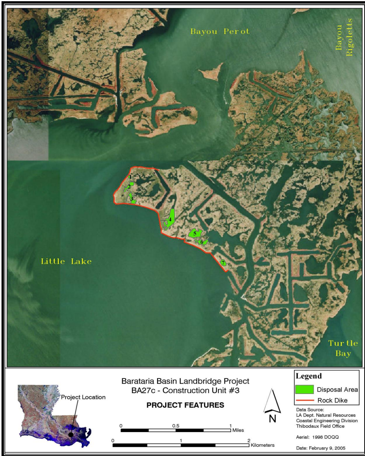
Figure 4. Project infrastructure map for the Barataria Basin Landbridge Shoreline Protection Project (BA-27c) – Phase 3, Construction Unit 3.
