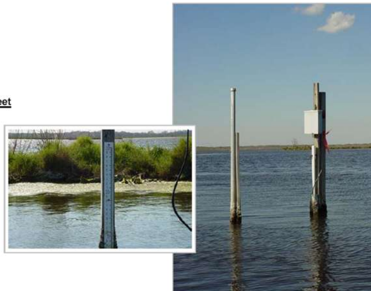
Position determined by using Real-Time Kinematic (RTK) survey from Secondary GPS Monument "FLOOD" Position established by T. Baker Smith & Son, Inc. for the Louisiana Department of Natural Resources, Coastal Restoration Division
