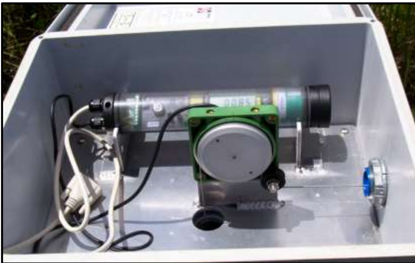
Figure 3.5b. Photograph of a typical static marsh mat continuous recorder station deployed in the field and of the Ott-Thalimedes data logger and pulley.
