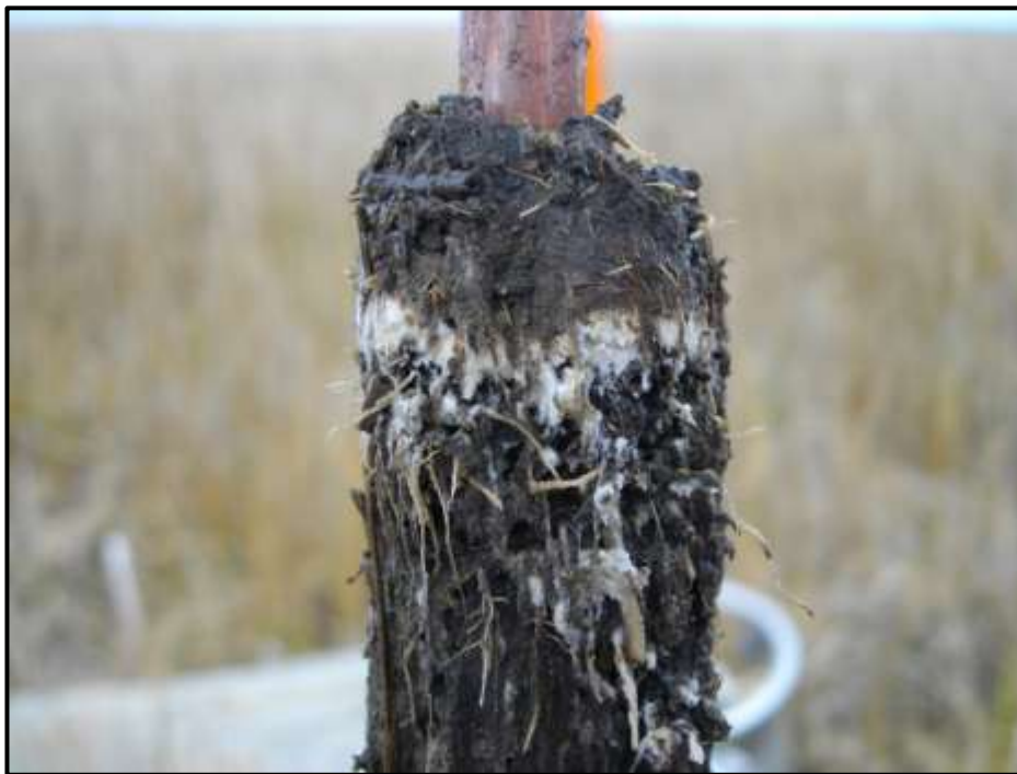
Figure 5.4. Photographs depicting accretion being measured above feldspar on a cryogenic core (top) and detail of a white feldspar ring on a frozen core (bottom).
