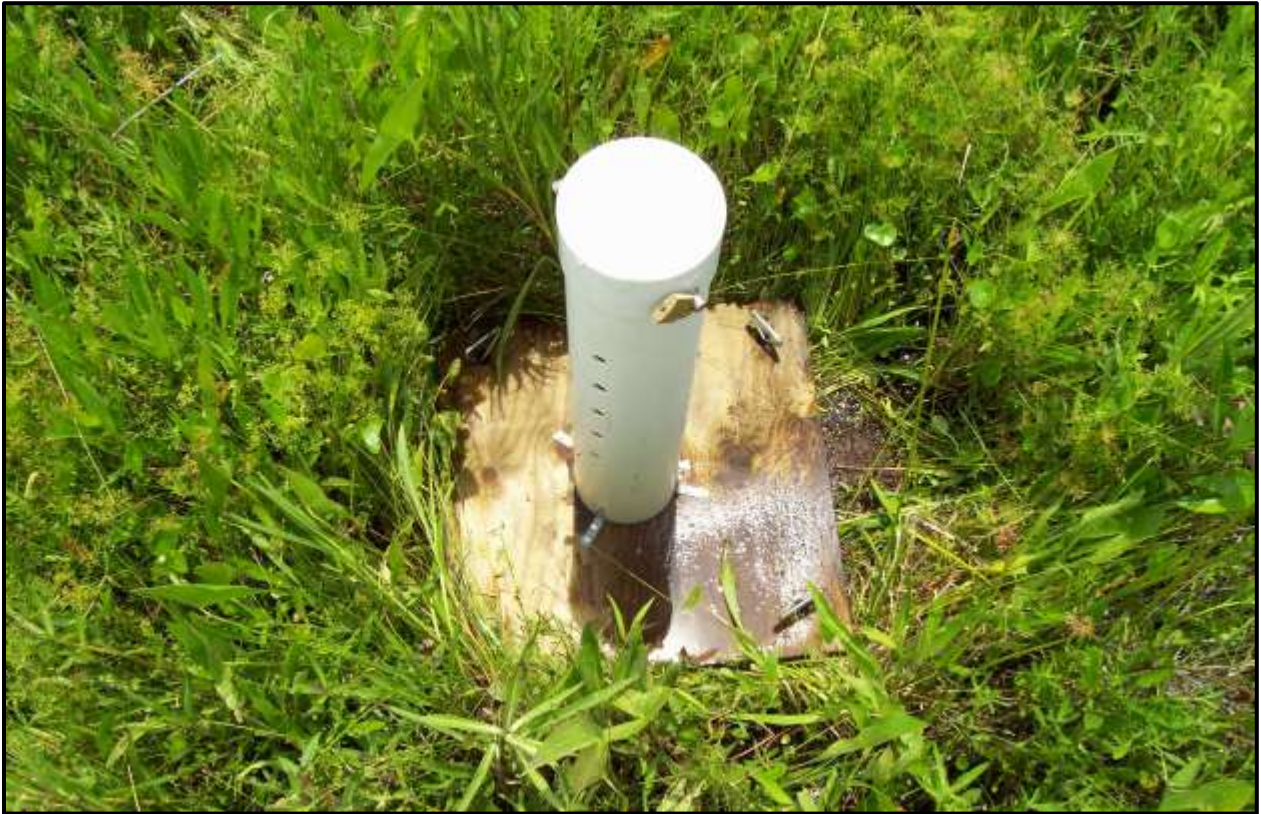
Figure 3.4b. Photograph of a typical floating marsh mat recorder deployed in the field.
