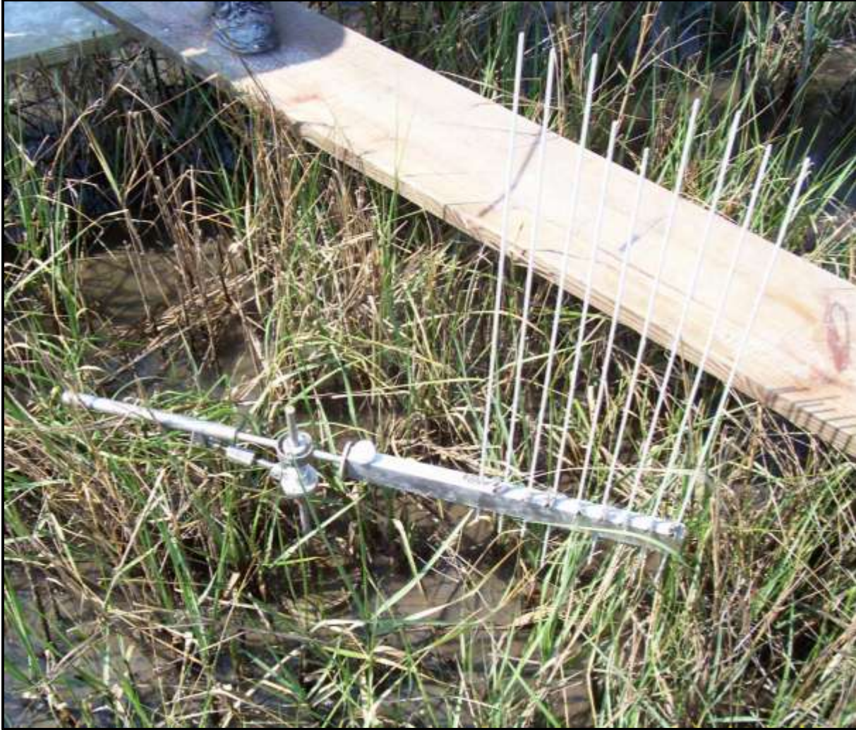
Figure 4.2b. Photograph of a RSET instrument with pins setup on the rod and collar prior to lowering the pins down on to the marsh surface.
