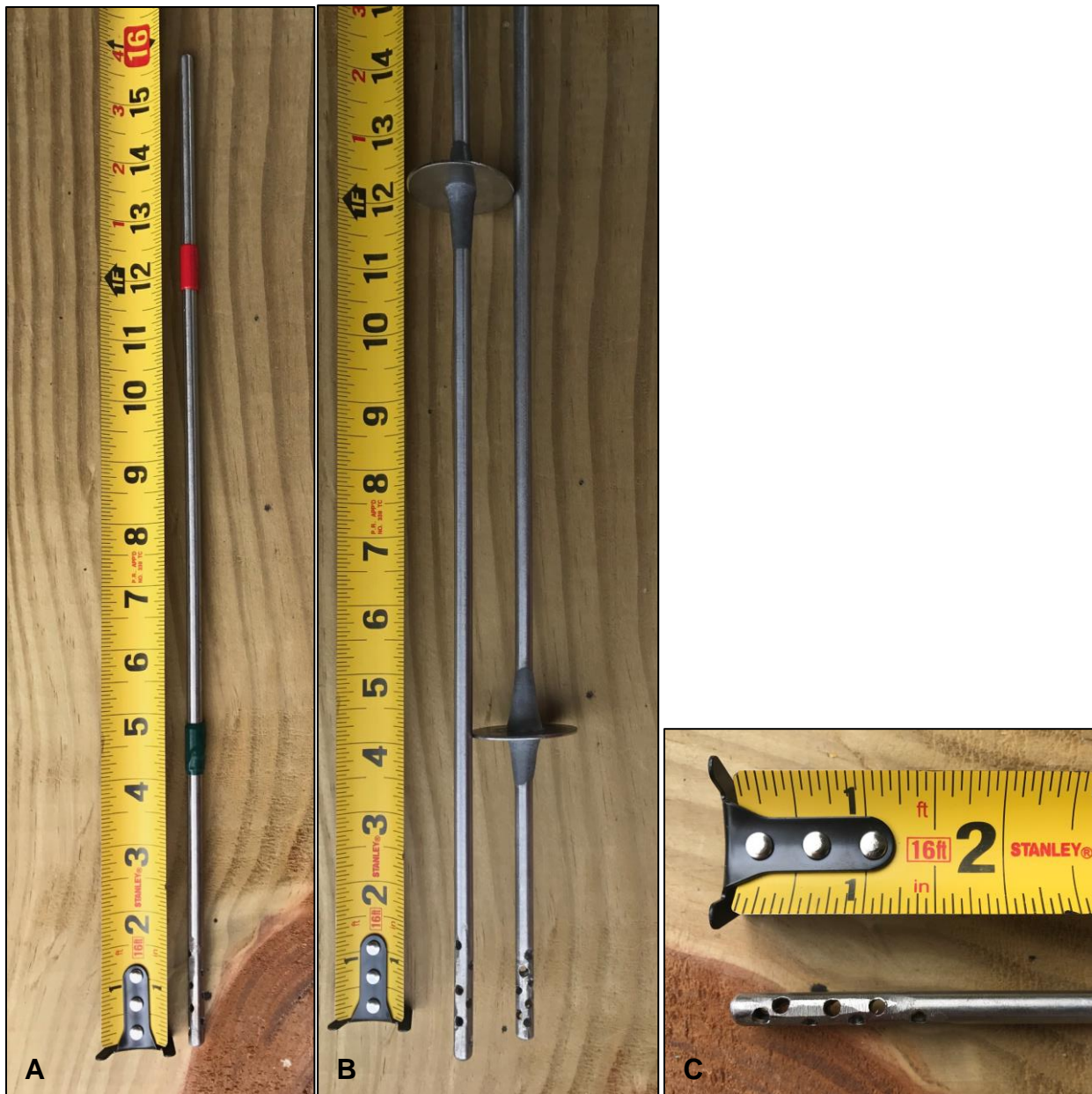
Figure 3.23. Stainless steel sipper tube alternatives for soil porewater collection. (A) Green and red tape mark 10 cm and 30 cm soil depths, respectively, for non-flooded conditions. (B) Metal washers fixed with a marine grade, metal adhesive (epoxy or weld compound) stop the tube at 10 cm and 30 cm soil depths in flooded conditions. (C) Larger diameter holes (1/8 in. diameter) are drilled to reduce clogging at the extraction depth.
