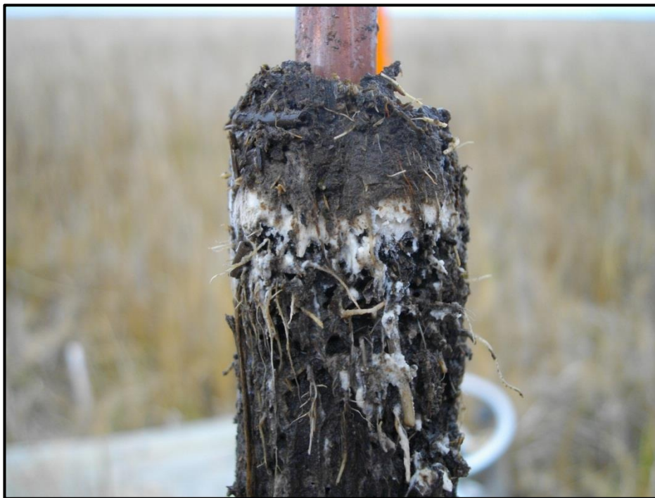
Figure 5.5. Photographs depict accretion being measured above feldspar on a cryogenic core (top) and detail of a white feldspar ring on a frozen core (bottom).
