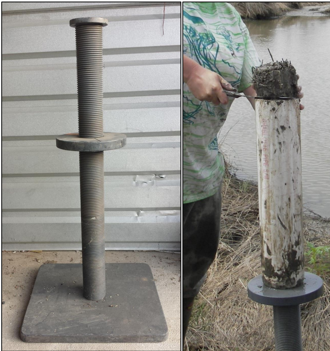
Figure 8.3b. Photographs of a core extruder (left) and a 4-cm core section being extruded and sliced in the field (right).
