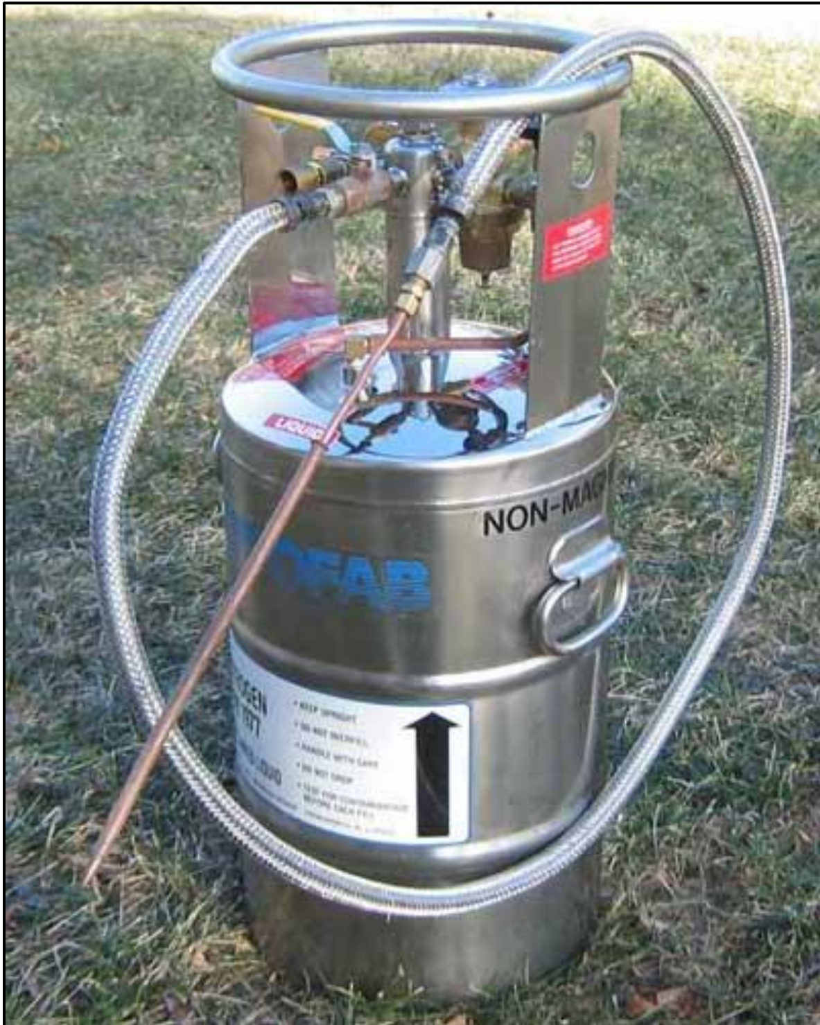
Figure 5.4b. Photograph of cryogenic coring equipment including the liquid nitrogen cylinder (cryo-cyl), flexible hose, and copper bullet (cryo-probe).
