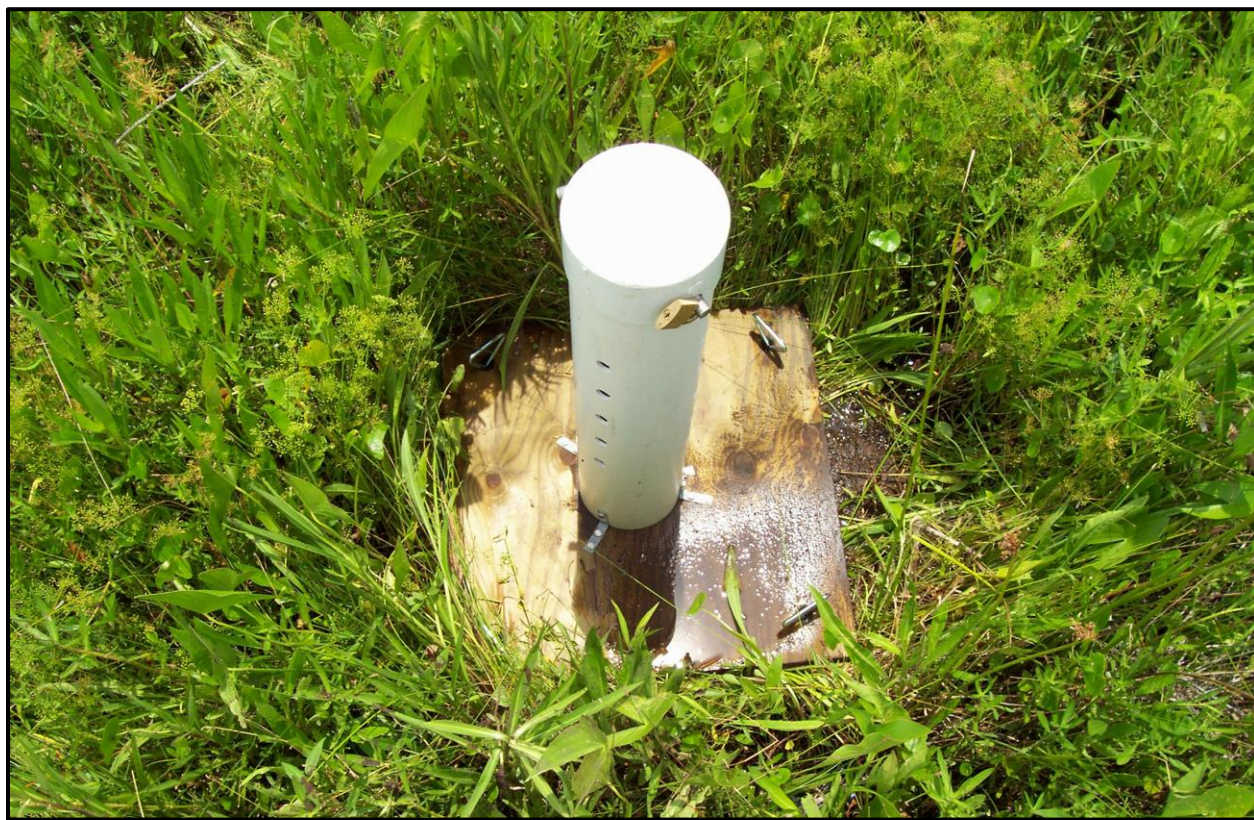
Figure 3.4b. Photograph of a typical floating marsh mat recorder deployed in the field.
