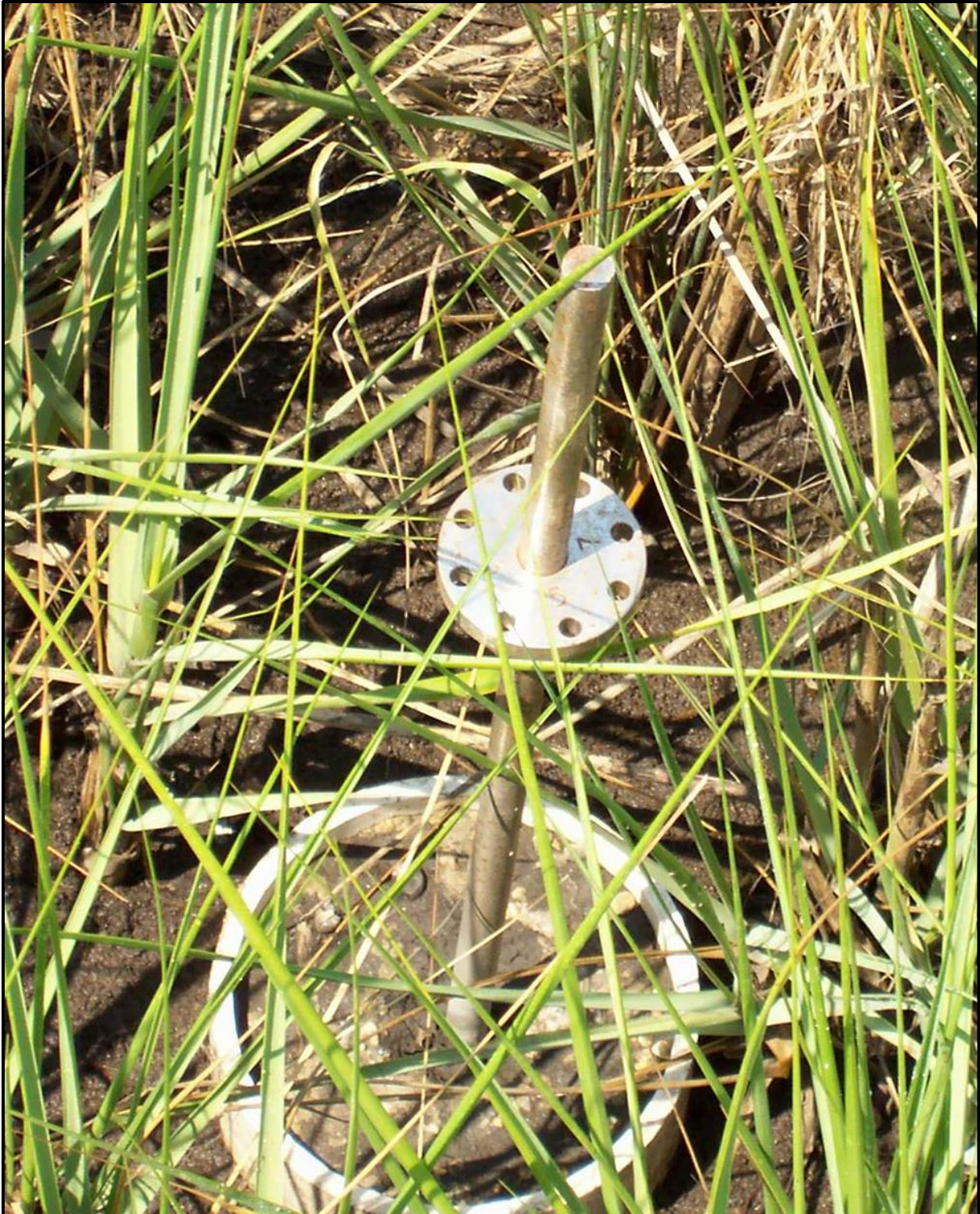
Figure 4.3b. Photograph of an RSET rod and collar installed in the marsh.
