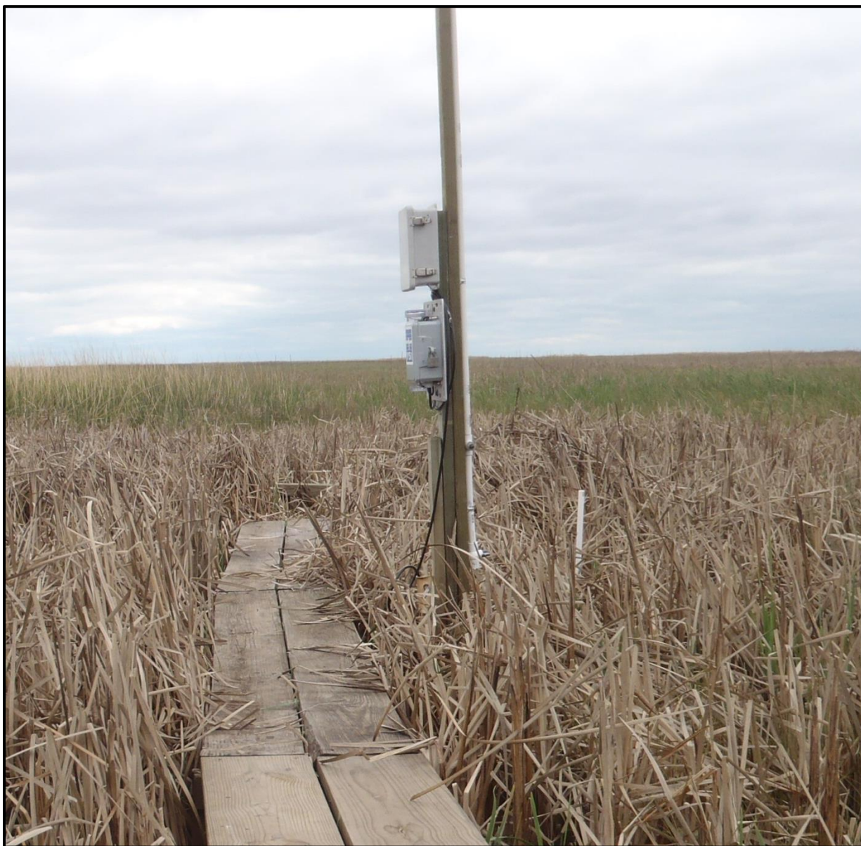
Figure 3.3b. Photograph of a marsh well station deployed at a boardwalk.
