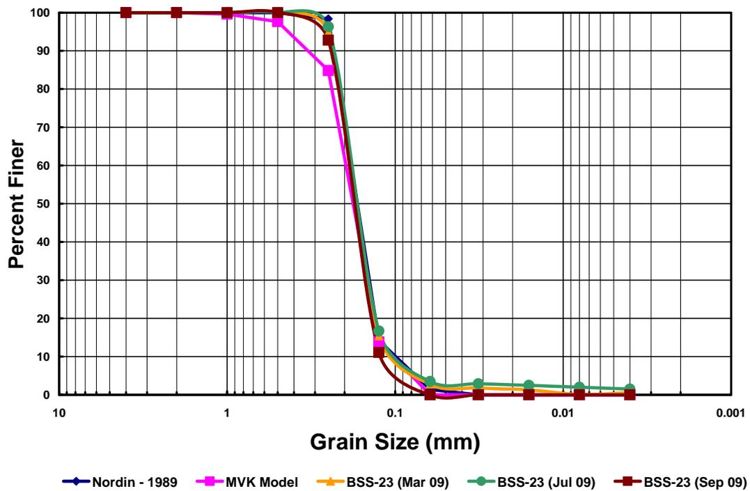
Figure 4.8. Bed Material Gradations At Site BSS-23
