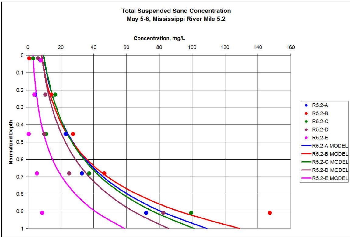
Figure 5.13. Suspended sediment verification at RM 5.2 for May 5-6.
