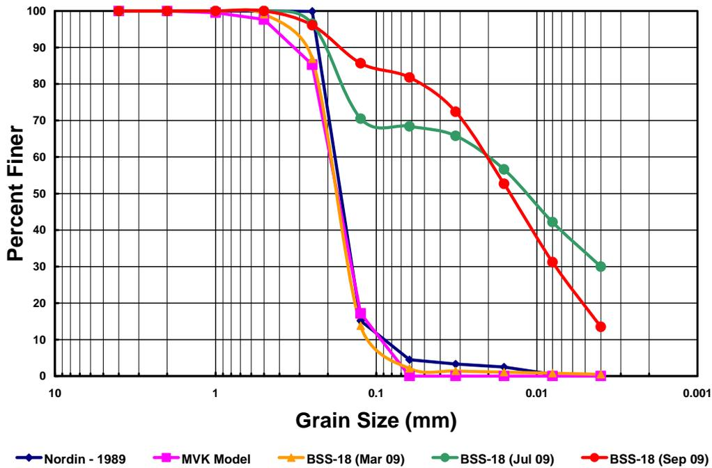
Figure 4.6. Bed Material Gradations At Site BSS-18
