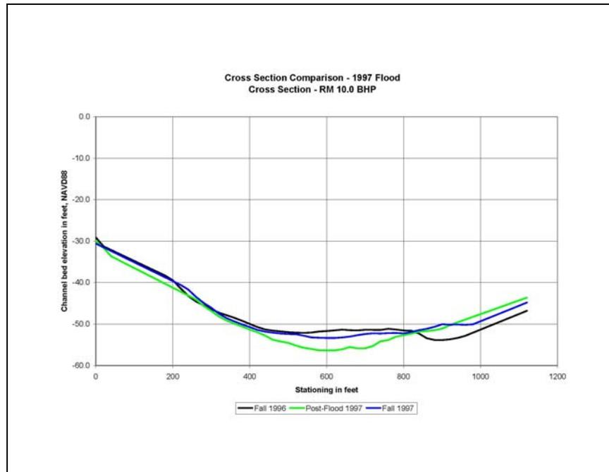
Figure 3.26. Cross section comparisons for 1997 flood for cross section located at RM 10.0 BHP.
