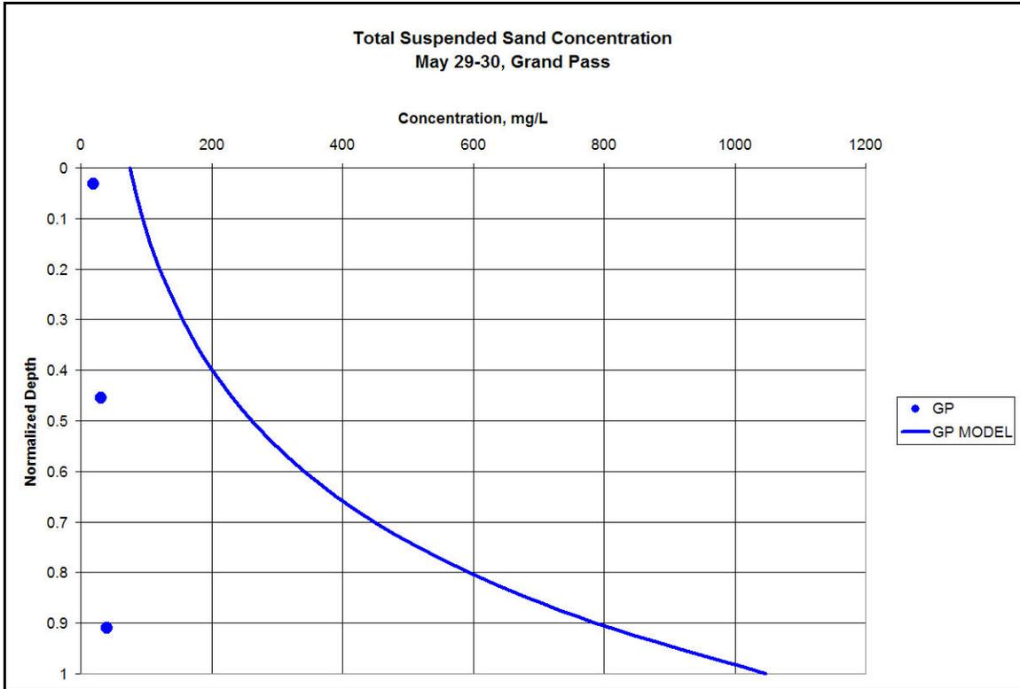
Figure 5.19. Suspended sediment verification at GP for May 29-30.
