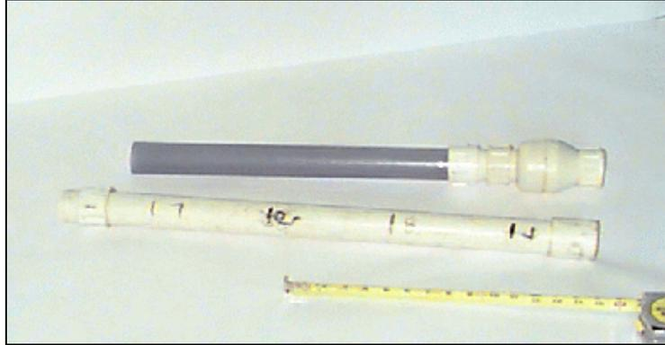
Figure 2.1. Push-core sampler.
