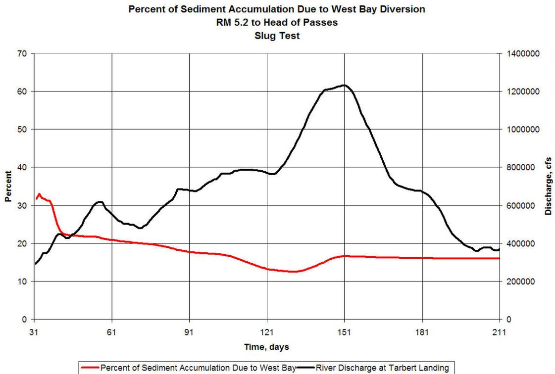
Figure 5.40. Percent increase in net deposition due to west bay diversion between RM 5.2 and Head of Passes, slug test.
