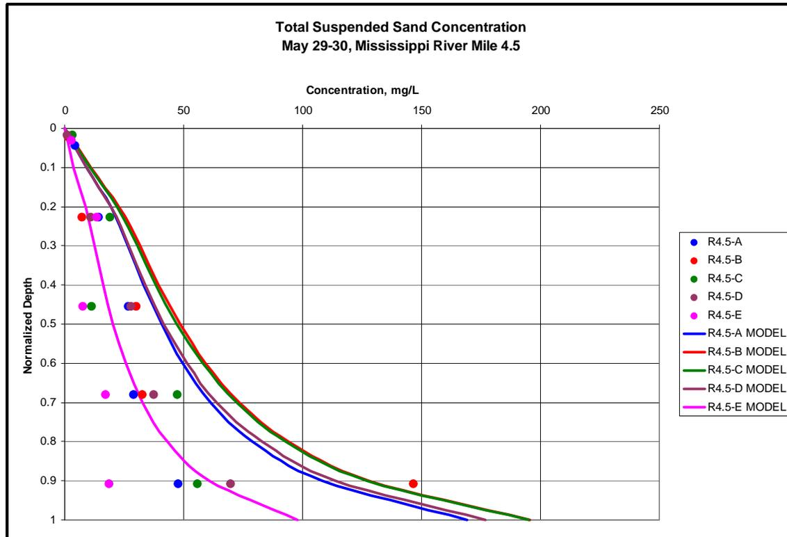
Figure 5.46. Sediment Concentration Comparison to Field Data, River mile 4.5.
