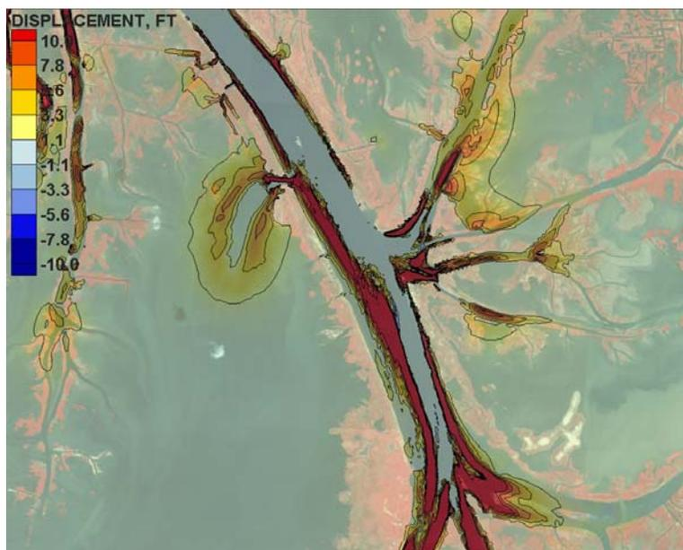
Figure 5.26. Cumulative bed change with West Bay Diversion, slug test run.
