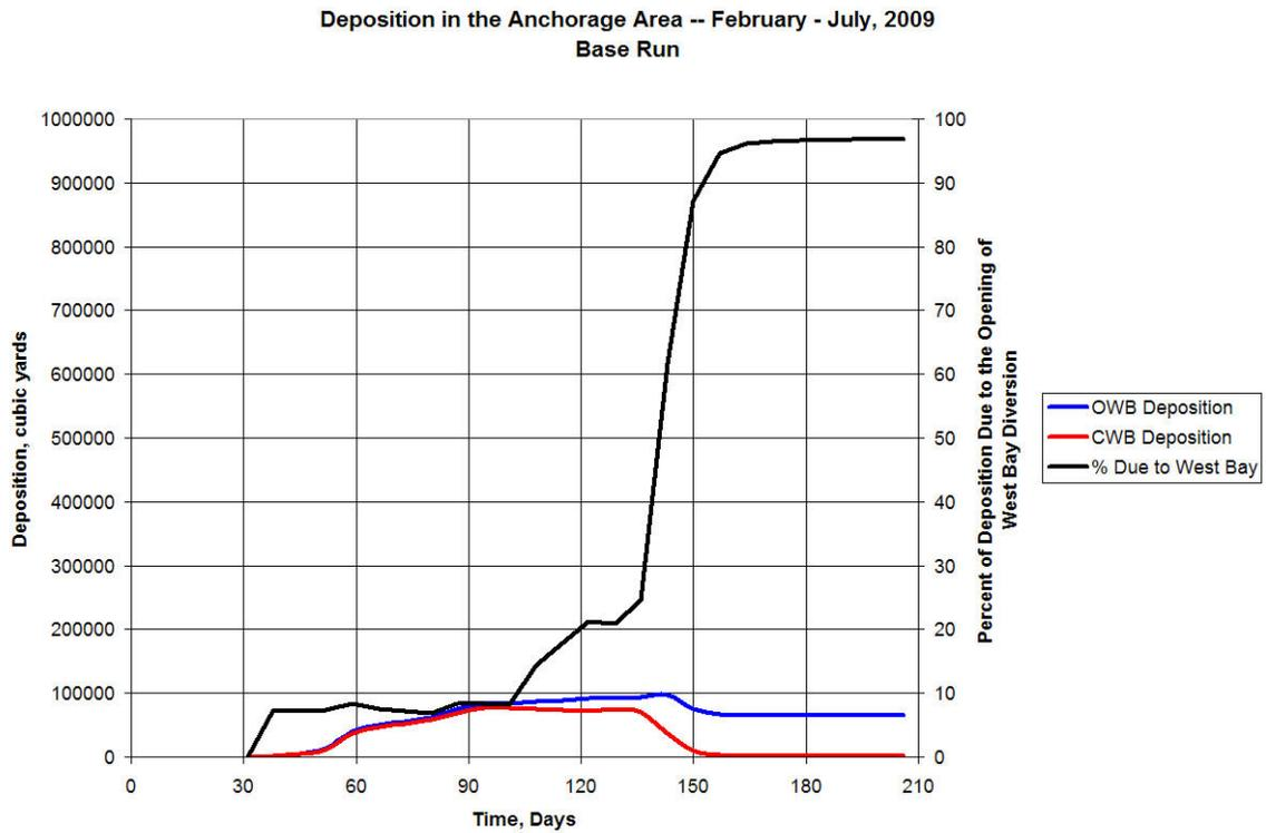
Figure 5.30. Deposition quantities for the anchorage area, base run.
