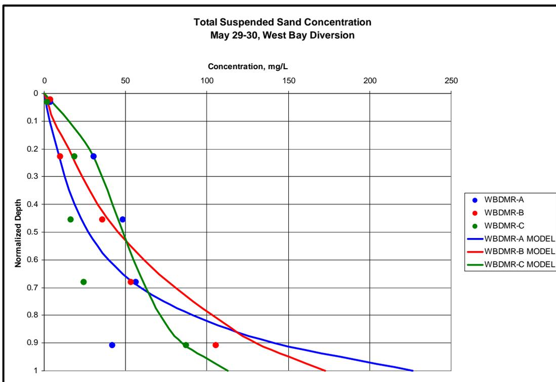
Figure 5.45. Sediment Concentration Comparison to Field Data, in Mouth of West Bay Diversion.
