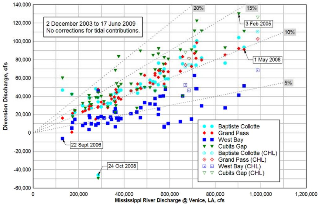
Figure 4.1. Measured Flow Distributions For Baptiste Collette Bayou, Grand Pass, West Bay Diversion, and Cubits Gap (2003 - 2009)
