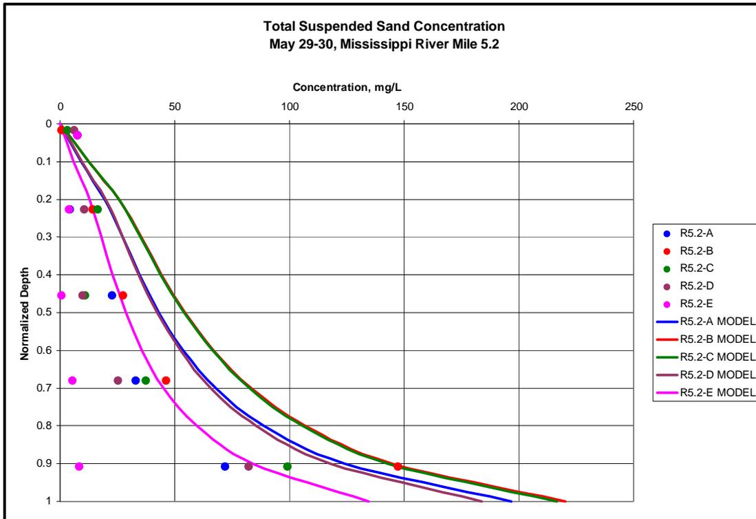
Figure 5.44. Sediment Concentration Comparison to Field Data, River mile 5.2.
