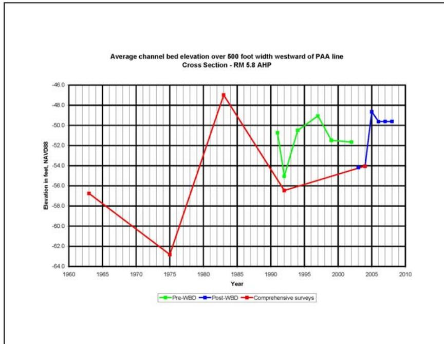
Figure 3.18. Comparison of average channel bed elevation for cross section located at RM 5.8 AHP.
