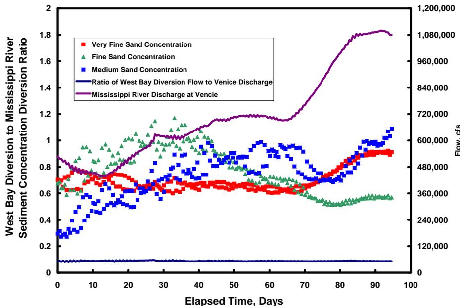
Figure 4.3. Estimated Sand Size Sediment Diversion Ratios for the West Bay Diversion Derived From the ADH 2-Dimensional Model
