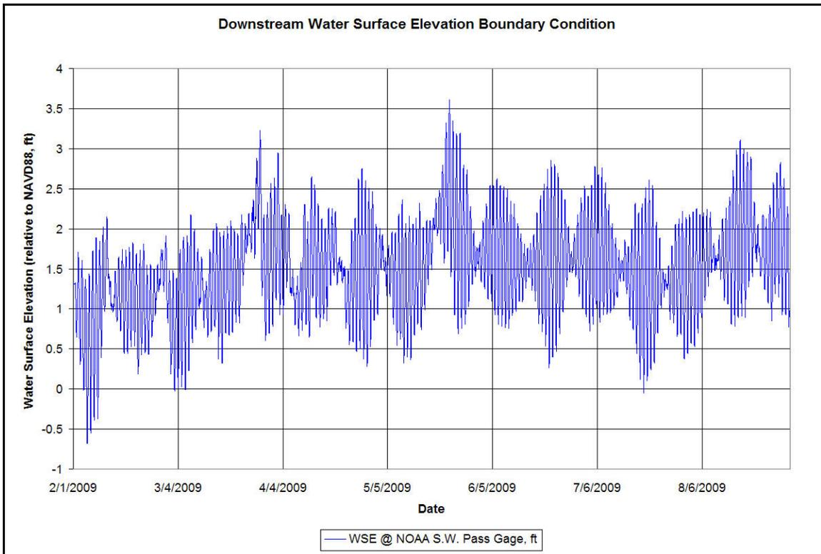
Figure 5.5. Downstream Water Surface Elevation Boundary for 2009.
