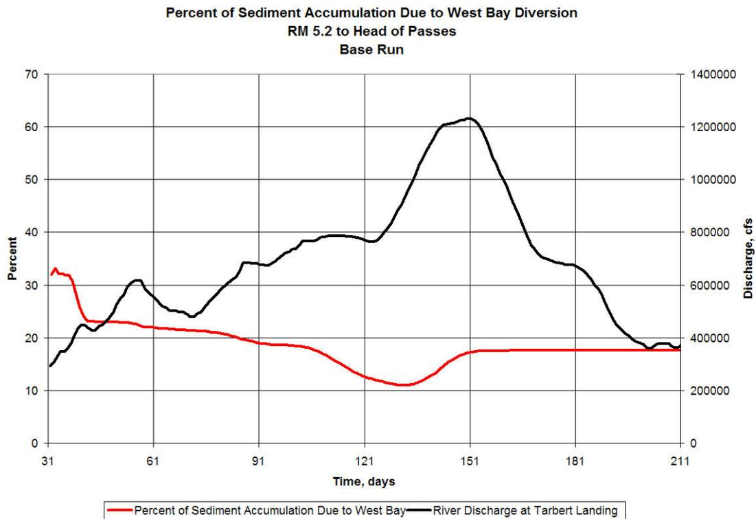
Figure 5.38. Percent increase in net deposition due to west bay diversion between RM 5.2 and Head of Passes, base run.
