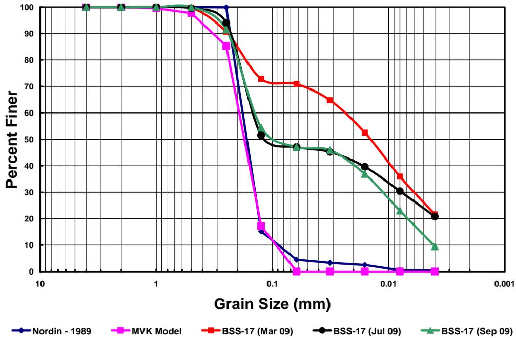
Figure 4.5. Bed Material Gradations At Site BSS-17
