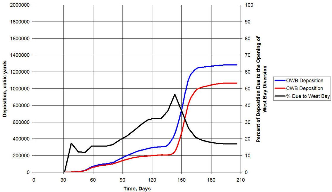
Figure 5.33. Deposition quantities for the adjacent channel, slug test.
