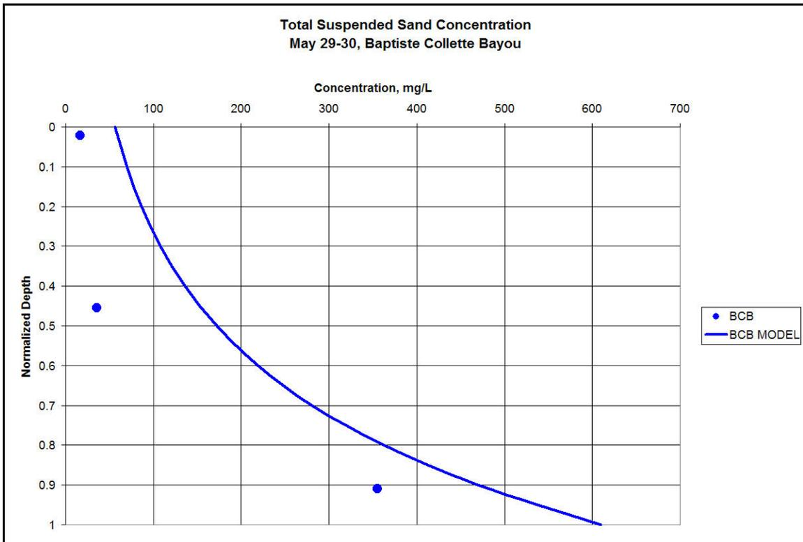
Figure 5.20. Suspended sediment verification at BCB for May 29-30.
