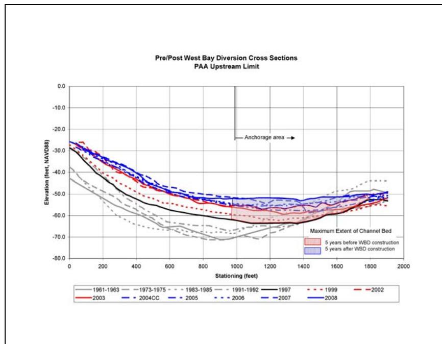
Figure 3.34. Maximum extent of channel bed elevation before and after West Bay diversion construction at upstream limit of anchorage area.
