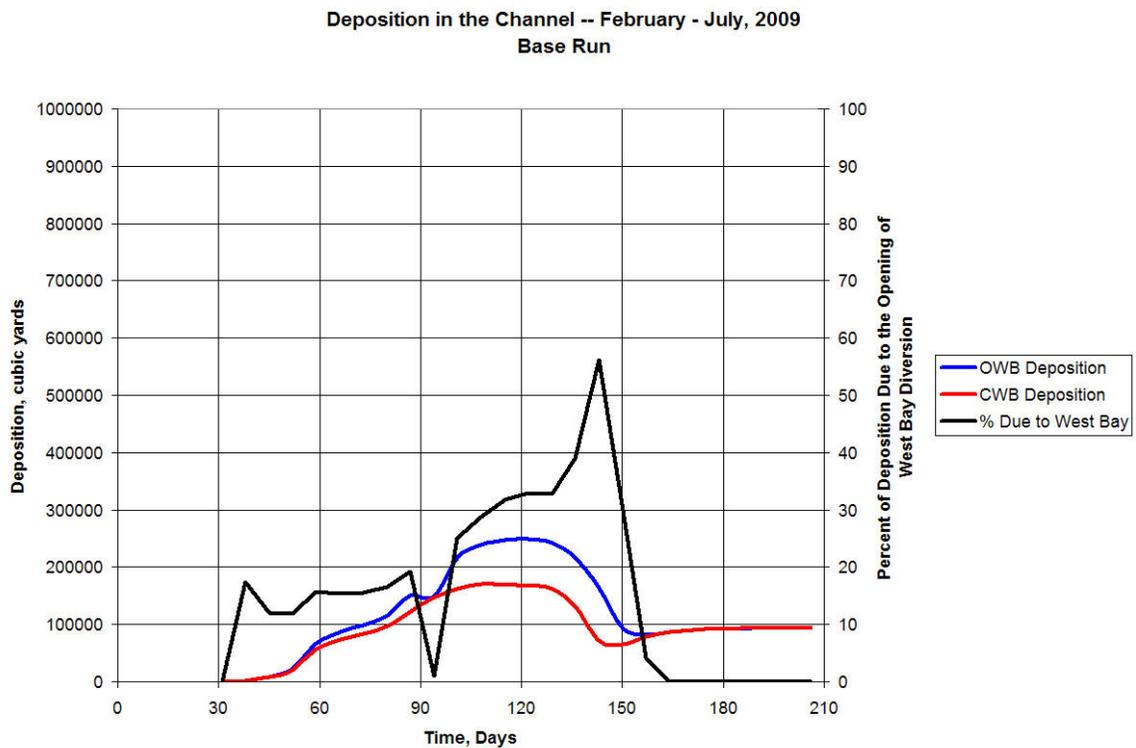
Figure 5.31. Deposition quantities for the adjacent channel, base run.
