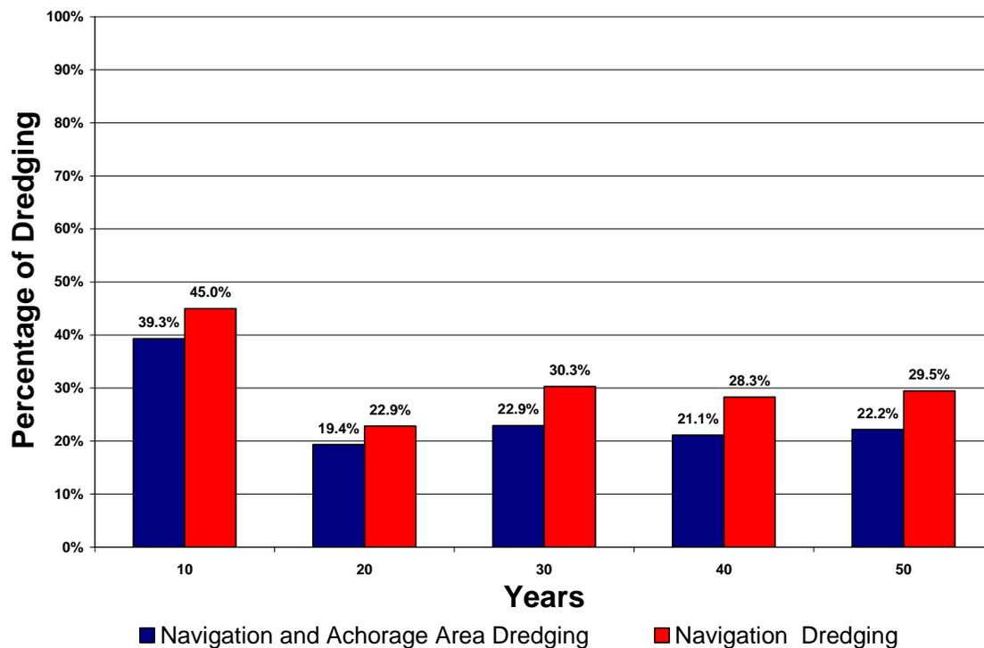
Figure 4.20. Percentage of Current Dredging Due to Opening West Bay Diversion
