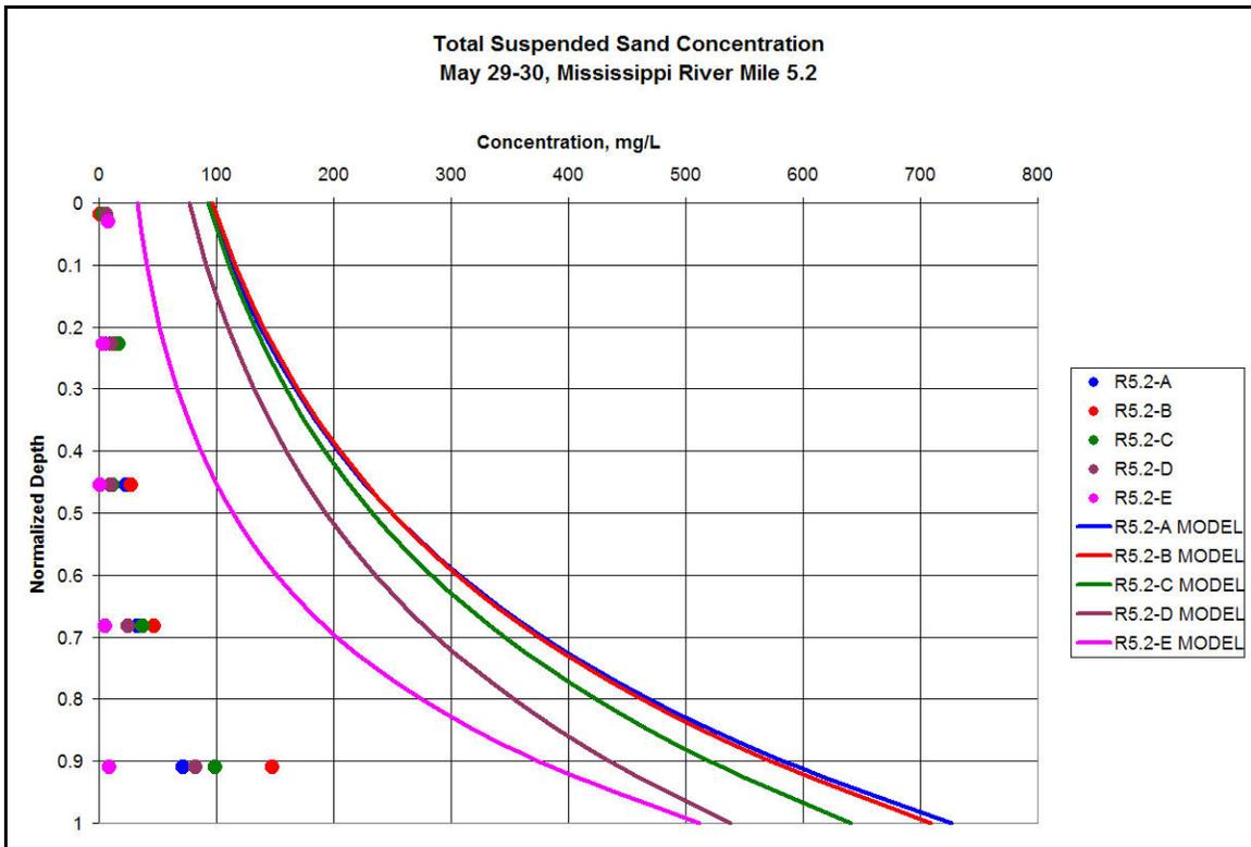
Figure 5.16. Suspended sediment verification at RM 5.2 for May 29-30.
