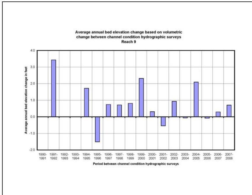
Figure 3.49. Annual average channel bed displacement between channel condition survey periods for Reach 9.
