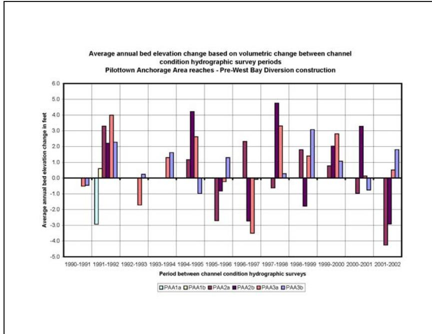
Figure 3.53. Average channel bed displacement based on pre-construction channel condition surveys for Pilottown anchorage area reaches.
