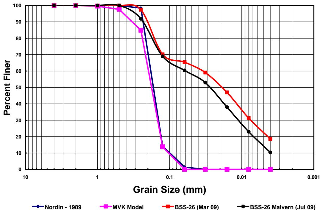
Figure 4.9. Bed Material Gradations At Site BSS-26
