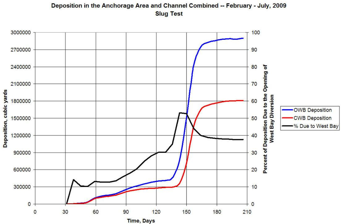
Figure 5.35. Deposition quantities for the combined anchorage area and adjacent channel, slug test.
