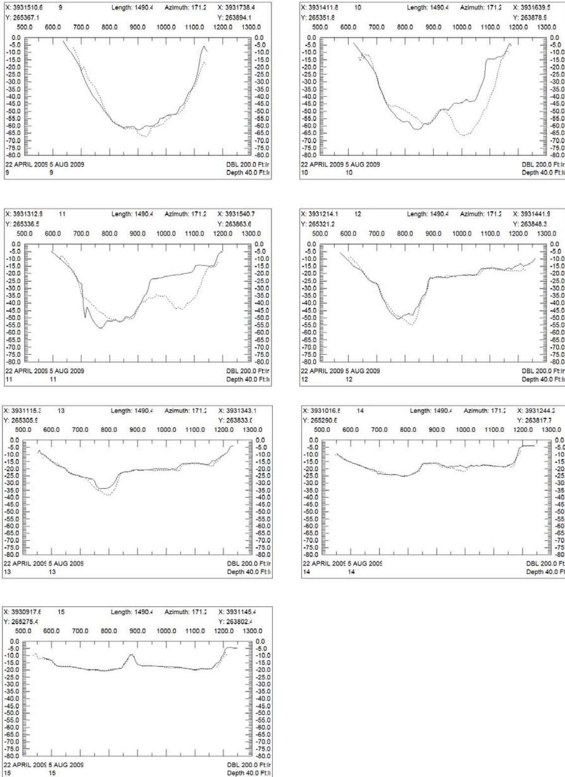
Figure 2.40. Cross sections of the Multi beam Survey Lines 9-15.
