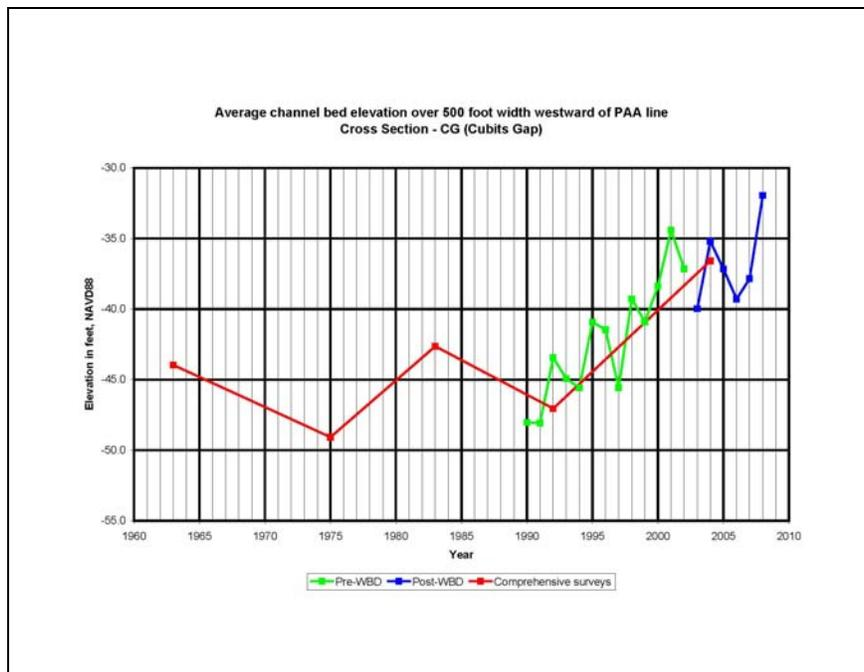
Figure 3.21. Comparison of average channel bed elevation for cross section located at Cubits Gap.
