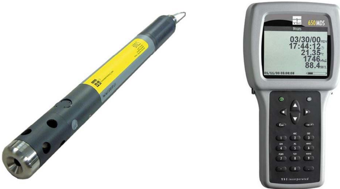
Figure 3.3: YSI 600LS Water Level Sonde (left) and YSI 650 Multiparameter Display System (650 MDS) (right) (YSI, 2017).
