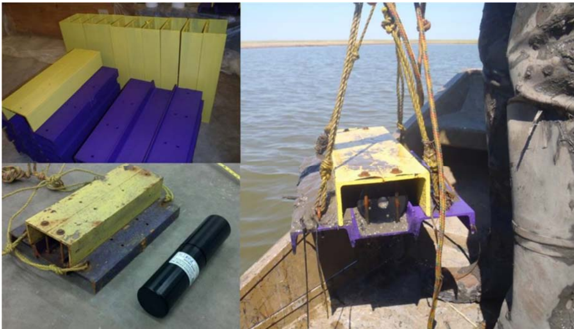
Figure 3.5: Fabricated baseplates (top left); assembled baseplate and OSSI-010-003C Wave Gauge (bottom left); wave gauge secured in baseplate housing (right) (Parker, 2014).
