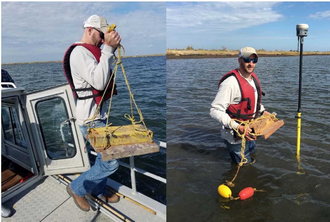
Figure 3.8: Deployment of Wave Gauge 505 (left) and Wave Gauge 502 (right) on 21 November 2017 (photo credit: (left) Navid Jafari, (right) Thomas Everett).
