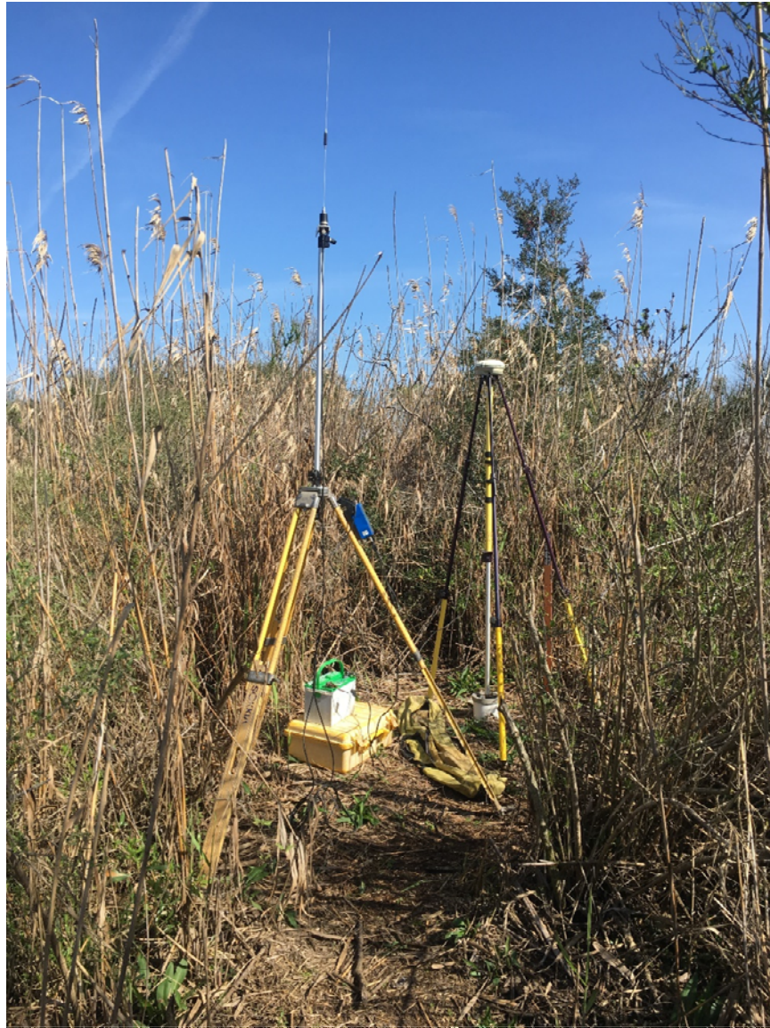
Figure 3.2: Setup of RTK GPS base station on secondary benchmark PO148-SM-01 on 14 February 2018.
