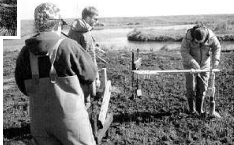
Project monitors shown here use the sediment erosion table technique to measure the accretion (build-up) of sediment in a project area. A flat table is suspended above the marsh surface and nine aluminum rods are inserted through it. Monitors measure the rate of sediment accretion as the distance between the table and the marsh surface decreases. (DNR photos)
