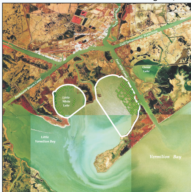
Four Mile Canal Terracing and Sediment Trapping (TV-18).
