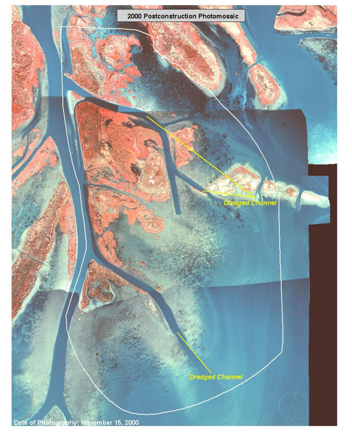
2,000 acres (809.4ha) of the delta. Natal Channel and Castille Pass are tertiary channels on the east side of East Pass. Each of these channels was dredged at an elevation of -10.0 feet (-3m). Construction for dredging began February 1, 1998 and ended on March 28, 1998.
