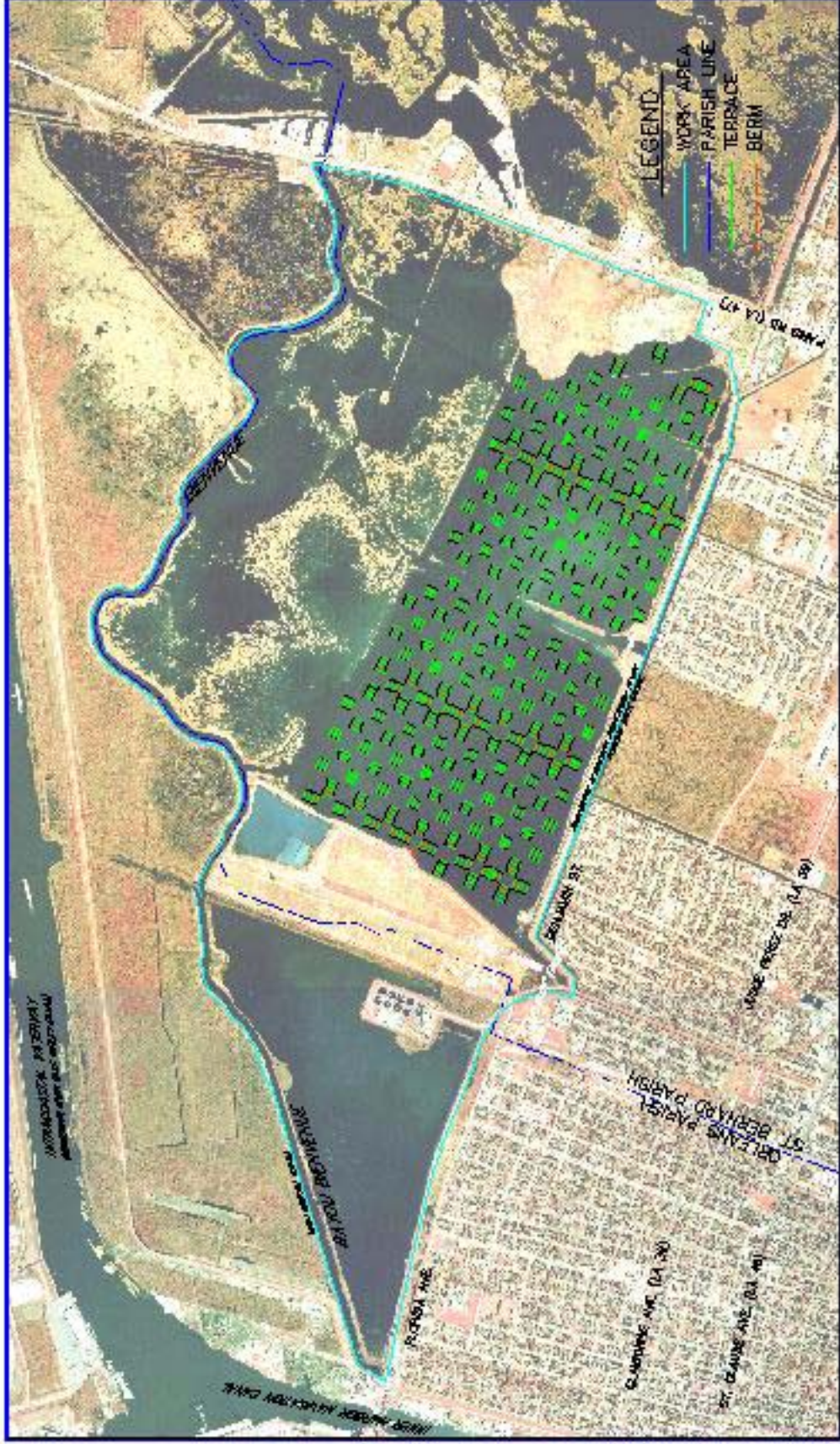
AERIAL LAYOUT SHOWING TERRACE ORIENTATION 3 APPROXIMATELY 41,000 LINEAR FEET OF TERRACES SHOWN IN CELL "B"
