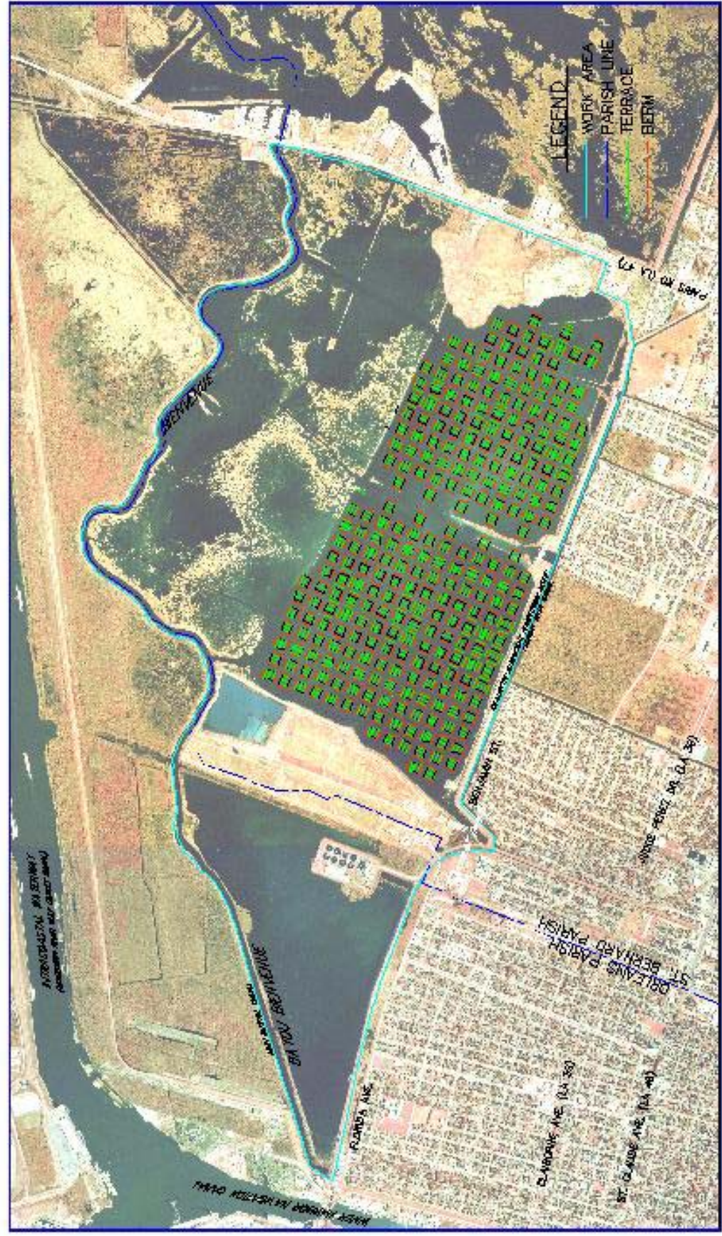
AERIAL LAYOUT SHOWING TERRACE ORIENTATION 2 APPROXIMATELY 95,000 LINEAR FEET OF TERRACES SHOWN IN CELL "B"
