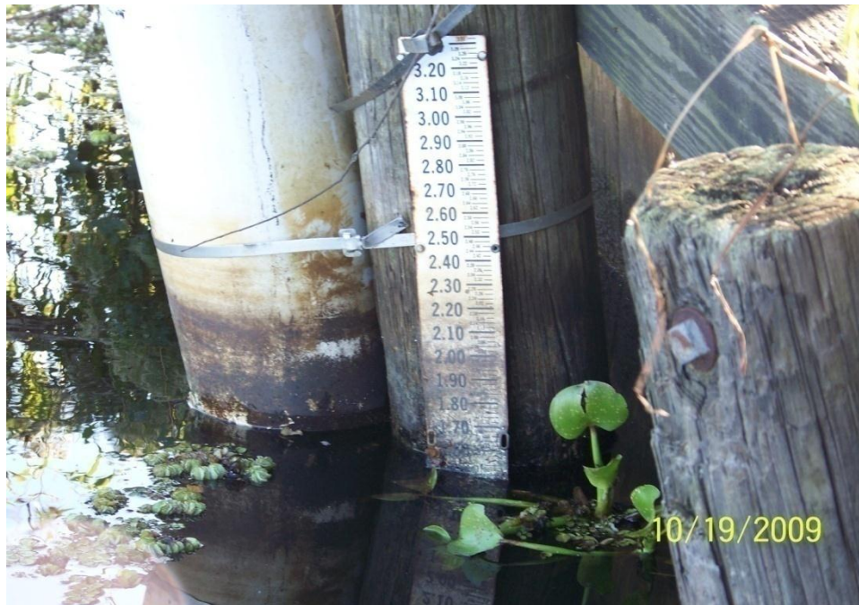
Photo No.1 –tide gage located along Minors Canal near the north bank of the GIWW.
