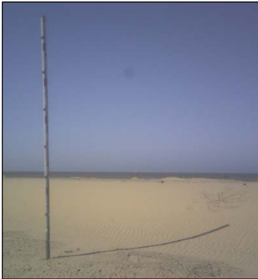
Figure 3: Photograph of a settlement plate on Shell West Barrier Island.
