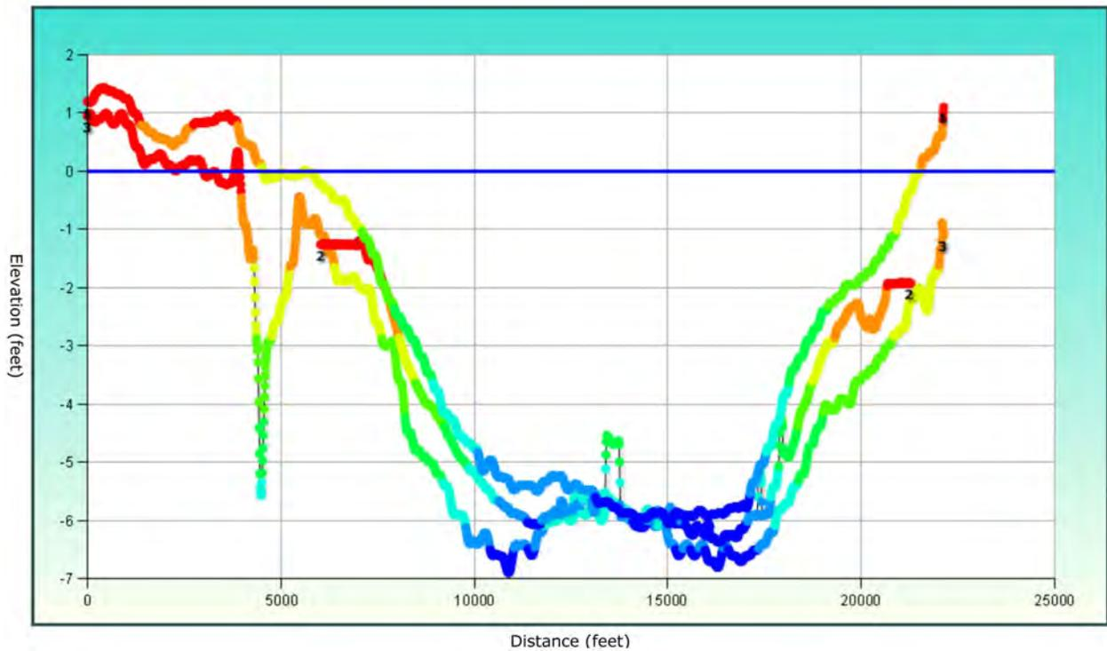
Figure 15: West Bay, Survey Cross Section Profile A-A (Produced by the Spatial Data Branch, Mobile District)
