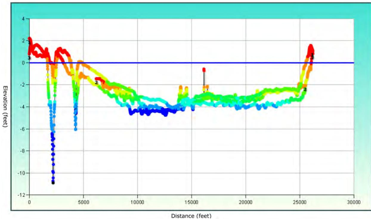
Figure 20: West Bay, Survey Cross Section Profile F-F (Produced by the Spatial Data Branch, Mobile District)
