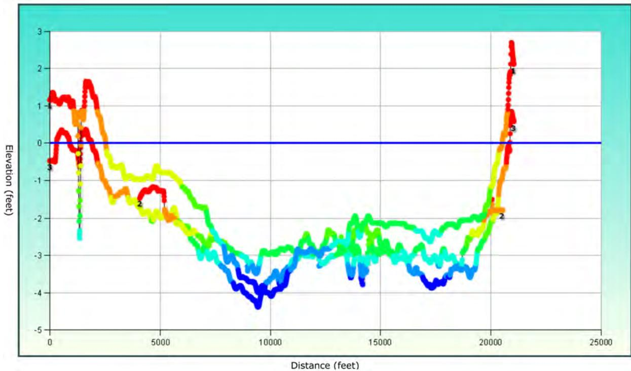
Figure 22: West Bay, Survey Cross Section Profile H-H (Produced by the Spatial Data Branch, Mobile District)
