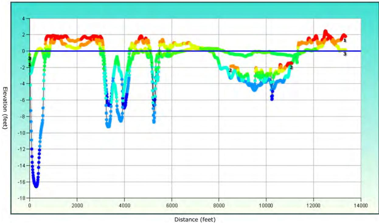
Figure 29: West Bay, Survey Cross Section Profile O-O (Produced by the Spatial Data Branch, Mobile District)
