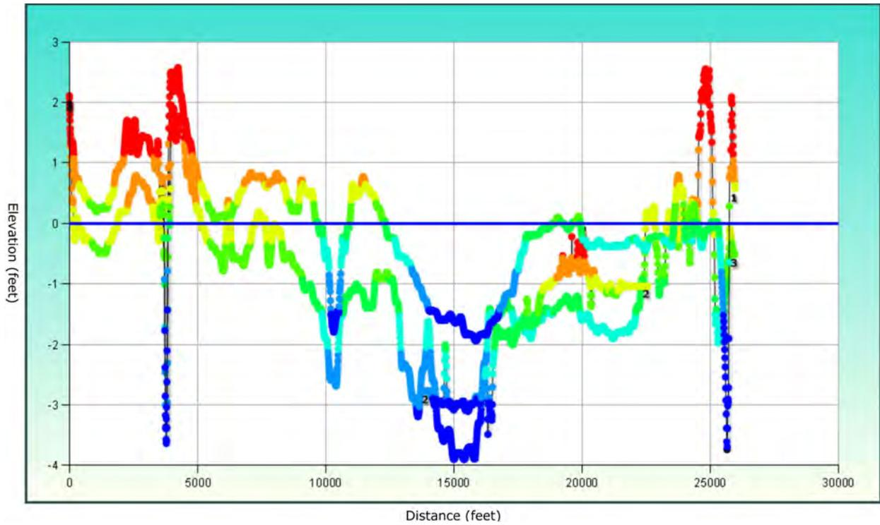
Figure 25: West Bay, Survey Cross Section Profile K-K (Produced by the Spatial Data Branch, Mobile District)
