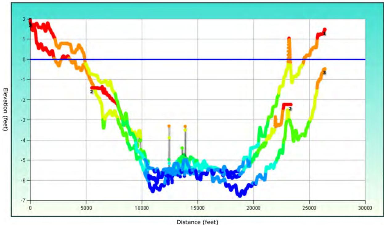
Figure 16: West Bay, Survey Cross Section Profile B-B (Produced by the Spatial Data Branch, Mobile District)
