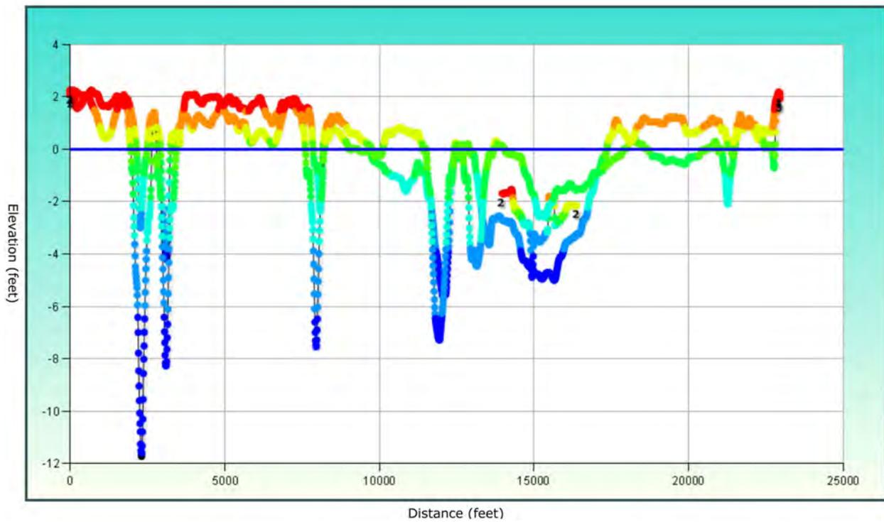
Figure 28: West Bay, Survey Cross Section Profile N-N (Produced by the Spatial Data Branch, Mobile District)
