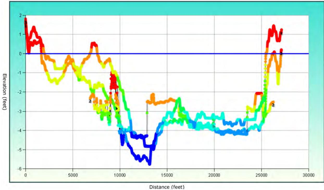
Figure 19: West Bay, Survey Cross Section Profile E-E (Produced by the Spatial Data Branch, Mobile District)
