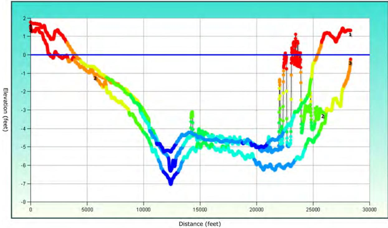
Figure 17: West Bay, Survey Cross Section Profile C-C (Produced by the Spatial Data Branch, Mobile District)
