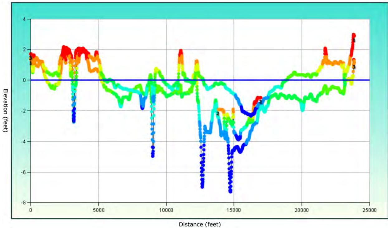
Figure 26: West Bay, Survey Cross Section Profile L-L (Produced by the Spatial Data Branch, Mobile District)
