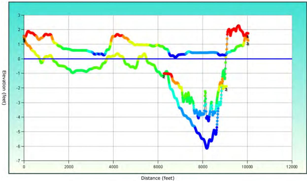
Figure 30: West Bay, Survey Cross Section Profile P-P (Produced by the Spatial Data Branch, Mobile District)
