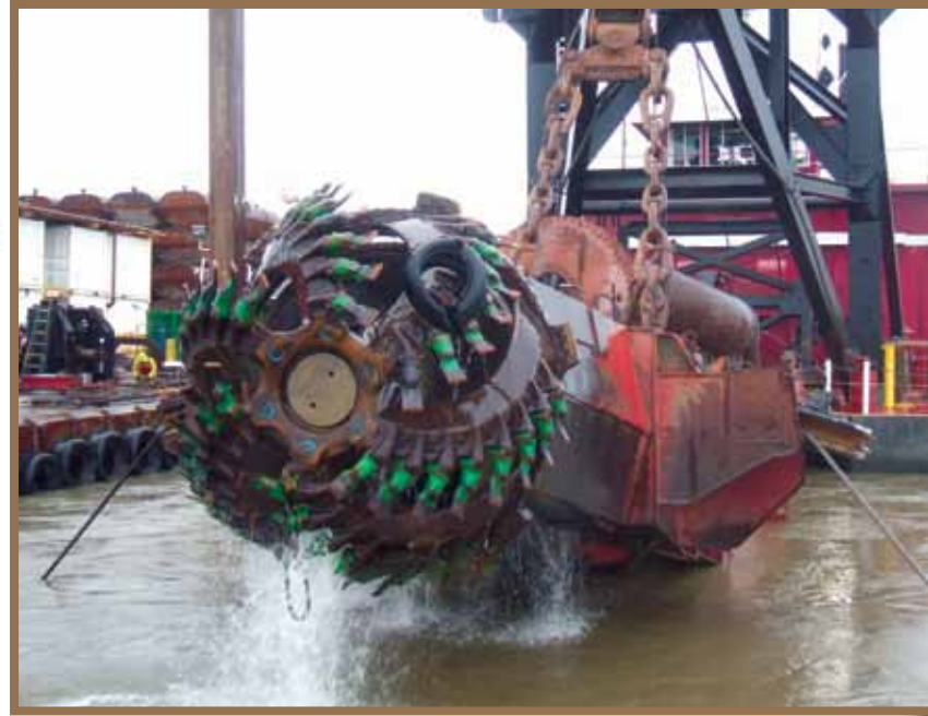
Hydrologic cutterhead dredge head. This dredge brings sediment from the river bed.
