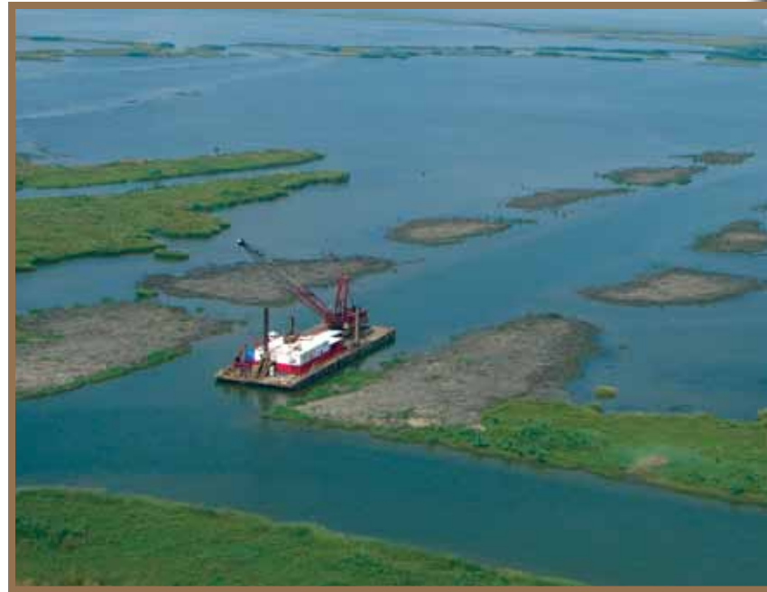
An artificial crevasse (gap) in the containment system allows for the diversion of fresh water and sediments.
